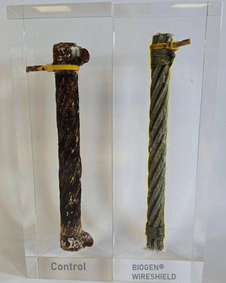
After 4000 hours of salt spray testing
